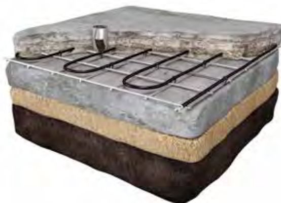
Installatie in beton
